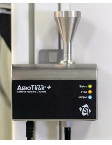
for a short time. However, the counter is not designed to resist high concentrations of VHP passing though the optics, which will quickly degrade and ultimately damage the sensor.
