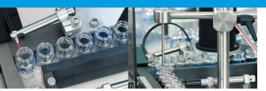
FF20 is a rotary vial/bottle handling system designed for use with Watson-Marlow Flexicon's liquid filling program, which encompasses both peristaltic liquid filling systems and a cream filler.
