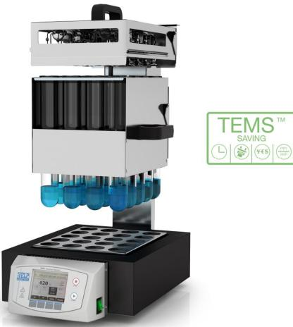
VELP digestion/mineralization systems are developed for different applications, from the determination of nitrogen and protein according to the Kjeldahl method (TKN) in food analysis to environmental analyses (Chemical Oxygen Demand) and chemical-pharmaceutical applications.
